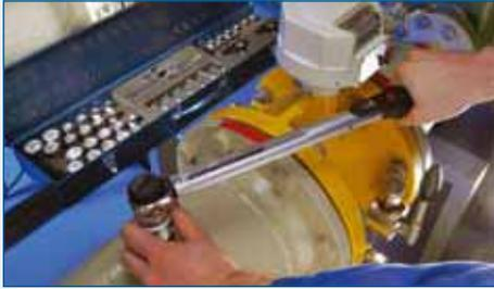
Working accuracy: +/- 3% tolerance of scale set torque. Includes test certificate according to DIN EN ISO 6789. Serial number on the wrench and on the certificate for unambiguous product identification, traceable to national standards.
