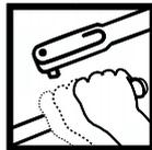
► Regardless of where you apply the force, at the center of the handgrip or another part of the DREMOMETER, with both hands or using an extension ube, your torque setting will always be attained, without shifts in value.
