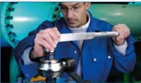
Safety: Torque multipliers starting from a ratio of 1:5 are fitted with anti-wind-up ratchets.
